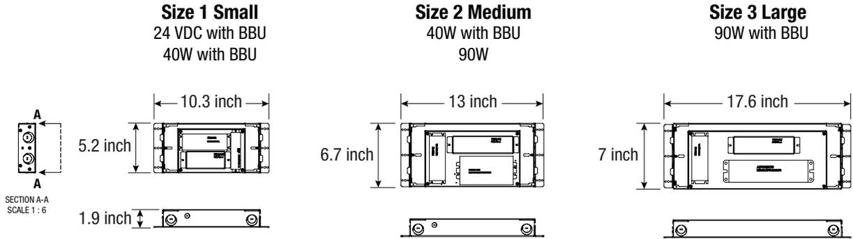
**BBUX** — Battery Backup & LED Driver Remote (Outdoor), IP67, IK10, NEMA 4X, -20 to 55 °C (-4 to 131 °F), 30 feet Maximum Distance with 12AWG (with UNV Option Only)
